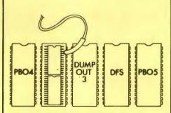
This new unit from Watford, which utilises the latest in Static RAM technology, offers 16k of easy-fit sideways RAM in a very compact unit with a footprint no larger than a standard 28pin EPROM. With only a single flying lead terminating in a mini hook-on probe, to fit, (no soldering required) this compact unit works with any BBC Micro with or without a ROM board.
